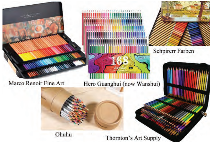
Deborah purchased five sets of inexpensive pencils to test. Fading started after only one week of exposure and, after two weeks, many more had faded or changed color, with two colors disappearing altogether. 28% of the colors tested from each set exhibited severe color changes after only two weeks.
